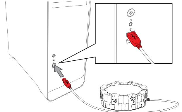
4 The Portal of Power interaction figure surface will illuminate when it is properly connected.
