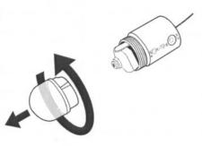
2. Adjust the focus by turning the lens.
