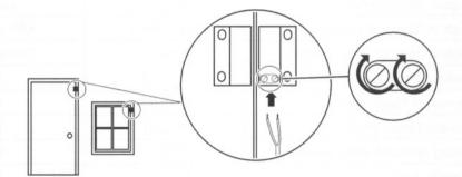
Insert the sensor cable wires into the reed switch and secure them by tightening the screws.
