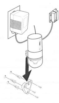
For soft materials such as wood skip to step 9. For concrete, brick, or stone surfaces, drill holes 23 mm deep with a 6-mm bit.
