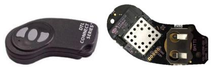
The DCR remote key fob uses the DTL02bluetooth radio to communicate to the DCC127 series photocontrol.
