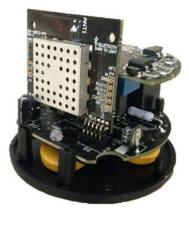
The DCC127 series photocontrol will use this DTL01bluetooth board in order to communicate to the keyfobDTL02.
