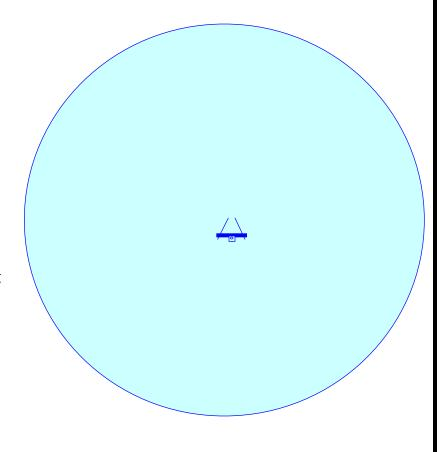
Side view, Omni Angle antenna coverage pattern. The coverage is elliptical with less coverage above and below the antenna than to the sides of the antenna.
