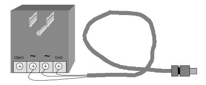
If available and/or needed, the reader may be powered by low voltage AC or DC power. This may be advantageous if there is other power sources available such a UPS or battery. The reader can operate with 10 to 18 VAC input or 10 to 24 VDC input. The power input pins are non-polarized and can be connected using either polarity DC. DC power may be useful if the reader is mounted in a remote location using a battery for power with a solar cell recharger to the battery.
