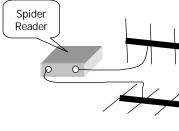
To cover the various orientations of the tag, two antennas at right angles to each other (one vertical and one horizontal). Aim both antennas at the same target area. egtenna is connected to one antenna connector on the Spider Reader.
