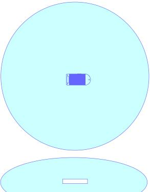
The transmission distance in the other plane of the tag is considerably shorter than the transmission distance of the primary plane.
