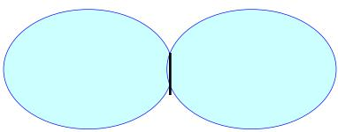
Side view, ¼ wave antenna coverage pattern. The view is looking at the side of the antenna. Coverage is a donut shape with less coverage above and below the antenna than on the sides of the antenna.
