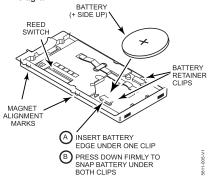
Mount 5811 using double-faced tape (supplied) by affixing it to the back of the unit and mounting the unit in place. Use screws (optional) if desired; see diagram. Mount the magnet (supplied) near the alignment marks on the case (see Diagram).
