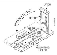
3. Engage the case tabs (see diagram), then rotate the housing to close. Engage latch with firm pressure to close and lock.
