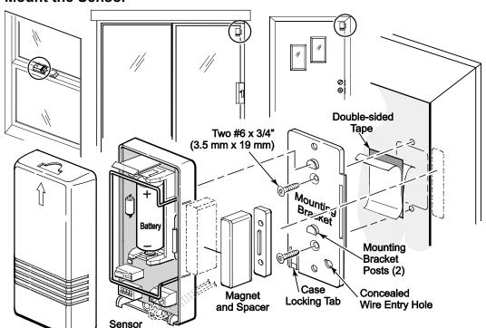
After enrolling and before mounting permanently, conduct Go/No Go tests (see the control's instructions) to verify adequate signal strength. Reorient or relocate the device if necessary.
