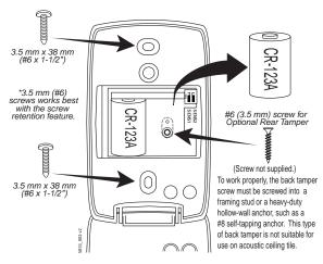
\*The screw retention feature simplifies installation: A rib in the screw cavity lightly holds the screw in place when installing the detector.
