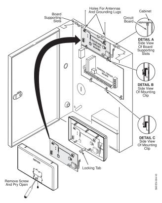
Figure 2. Installing the Receiver Board in Control's Cabinet
