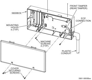
Figure 5: 5881ENHC UL Commercial Fire Installation
