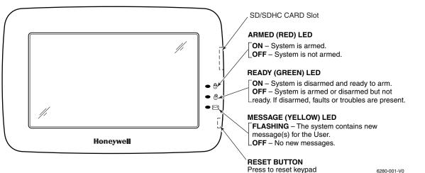
\*Note: If the EN50131 Display feature is enabled, the "Armed" and "Ready" status LEDs turn OFF after 30 seconds and the screen returns to the Home screen until a valid user code is entered.
