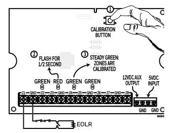
IMPORTANT! ONCE THE SIXC2W IS CALIBRATED, ANY CHANGE IN THE ZONE RESISTANCE THE MODULE MUST BE RE-CALIBRATED.
