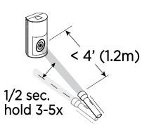
**Note**: the flashlight feature only initiates or restarts the Test Mode and does not change any other sensor settings.
