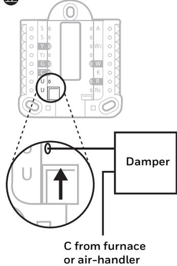
Wired to humidifier, ventilator, or damper powered by external transformer
