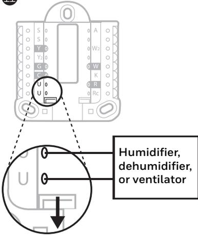
Wired to fresh air damper powered by furnace transformer.
