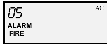
TYPICAL FIRE EMERGENCY DISPLAY
