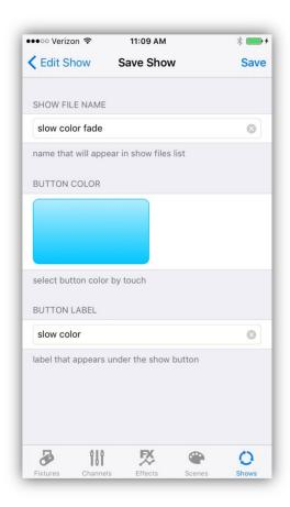
From this view you can enter a long descriptive file name for the show and a shorter name that will appear under the button in the Show buttons array. Touch and drag within the button view to change the button color. Tap the "Save" navigation button in the upper right to save the file. An alert will appear to confirm the save or to warn if another show is already using that name.
