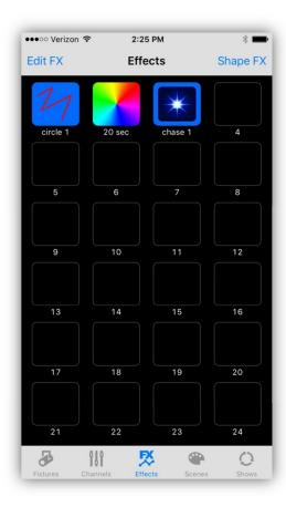
All three buttons in the example are highlighted indicating that all three effects are running. Tapping an effect button will toggle the effect on or off.
