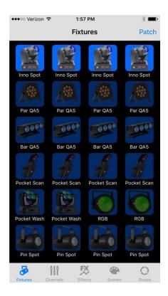
You will notice in this example that the top row of buttons is highlighted while the other rows are dimmed. This indicates that the top row has been selected for programming. Fixture selection is used to program the fixture channels as well as to program some of the effects.
