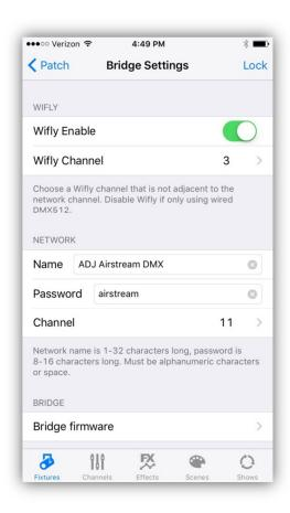
**Wifly Settings:** The top two rows are settings for the ADJ Wifly network. If you are using ADJ Wifly enabled fixtures, set Wifly Enable to on and set the Wifly channel to match the Wifly channel settings on your fixtures. Wifly supports channels 0-14. One of the example screenshots on the next page (right side) shows the view for setting the Wifly channel.
