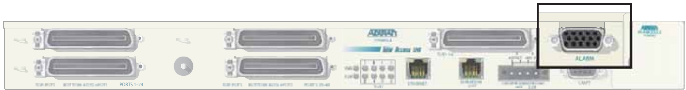
Figure 3-8. Total Access 1248 Alarm Connection
