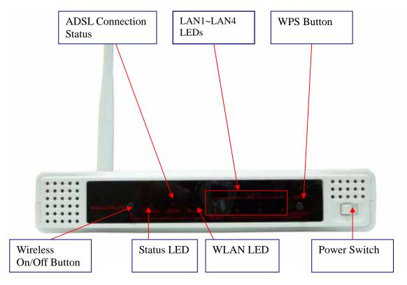
Reset: Press "Wireless on/off" and "WPS" button for 5 sec simultaneously.
