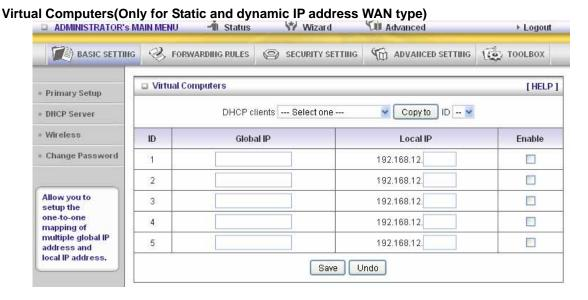
Virtual Computer enables you to use the original NAT feature, and allows you to setup the one-to-one mapping of multiple global IP address and local IP address.
