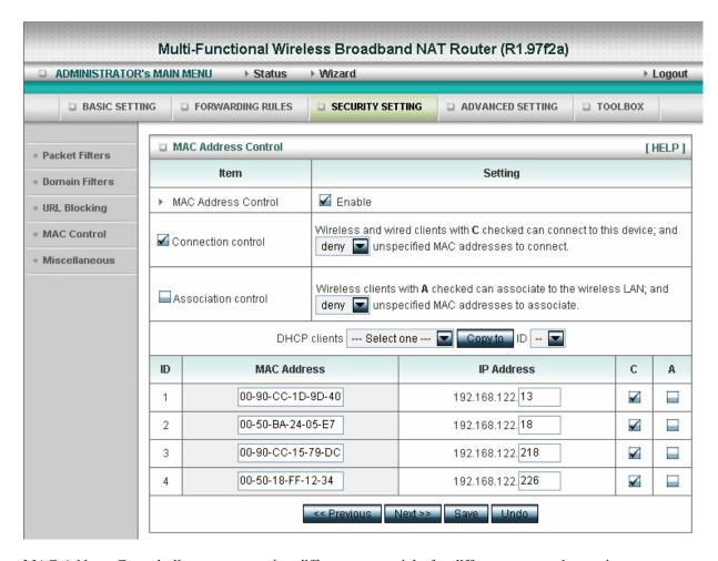
MAC Address Control allows you to assign different access right for different users and to assign a specific IP address to a certain MAC address.
