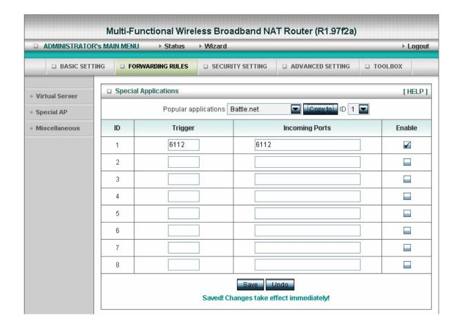
Some applications require multiple connections, like Internet games, Video conferencing, Internet telephony, etc. Because of the firewall function, these applications cannot work with a pure NAT router. The **Special Applications** feature allows some of these applications to work with this product. If the mechanism of Special Applications fails to make an application work, try setting your computer as the **DMZ** host instead.
