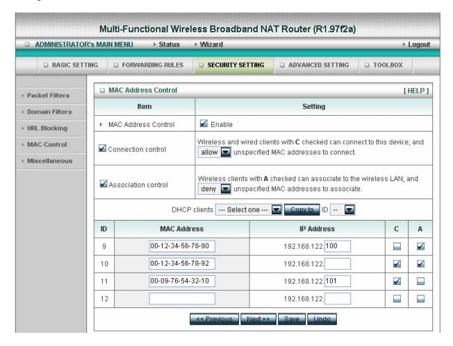
In this scenario, there are three clients listed in the Control Table. Clients 1 and 2 are wireless, and client 3 is wired.
