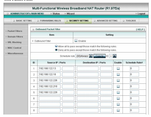
Packet Filter enables you to control what packets are allowed to pass the router. Outbound filter applies on all outbound packets. However, Inbound filter applies on packets that destined to Virtual Servers or DMZ host only. You can select one of the two filtering policies:
