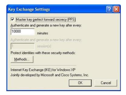
enable "Master key perfect forward security (PFS)" configure "Authenticate and generate a new key after every [10000] seconds" click [Methods...]
