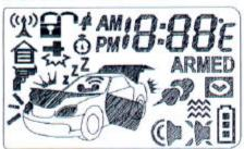
The LCD screen on the Remote control displays graphic icons or Figures. It provides you visual information on any trigger of the Sensors and around-a clock surveillance to your armed vehicle as well as showing the present status of the system.
