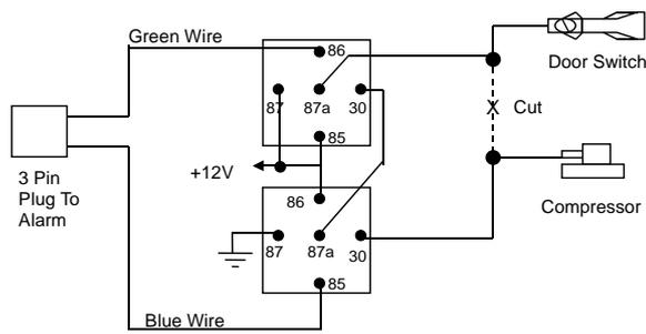
**2 STEP DOOR UNLOCK WIRE CONNECTION FOR 5 WIRE ALTERNATING DOOR LOCKS**
