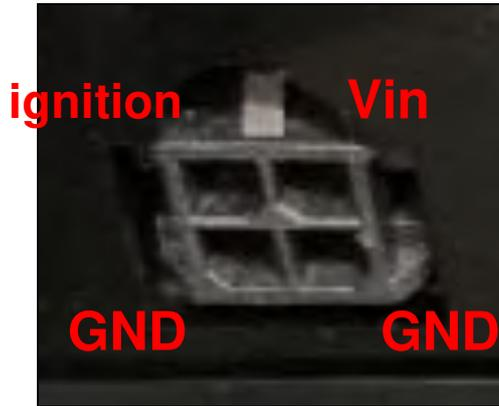
**Figure 9:** Ignition Sense Pinout
