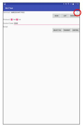
Remark: Select ICC for reading contact card while select PICC for reading contactless cards
