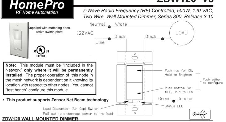
The ZDW120 Wall Mounted Dimmer is a component of the HomePro lighting control system. Wire the Wall Mounted Dimmer in place of the standard wall switch according to the diagram above and program from the Wireless Controller to operate loads. Inclusion of the ZDW120 Wall Mounted Dimmer on the ZTH100 Wireless Controller menu allows remote ON/OFF control and dimming of lights connected.
