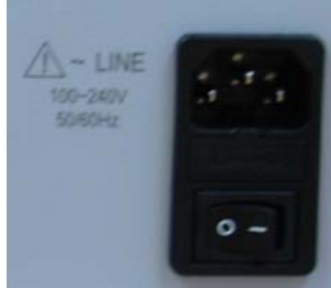
Figure 5 – ADRF-25K Repeater Power Switch View
