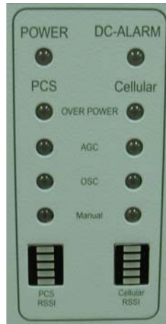
Figure 4 – ADRF25K Repeater LED View
