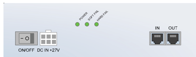
Figure 3-43 Ports at the rear panel (Slave RU)
