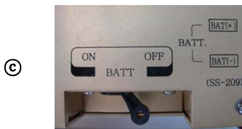
Figure 7: Battery Select Switch
