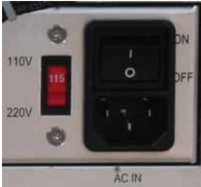
Figure 3: Axiom Repeater Power Switch View
