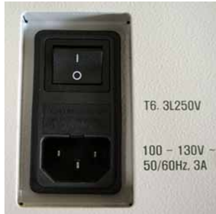
Figure 1: AXM700 Repeater Power Switch View
