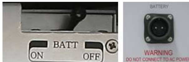
Figure 9 – Battery Switch & Battery Port
