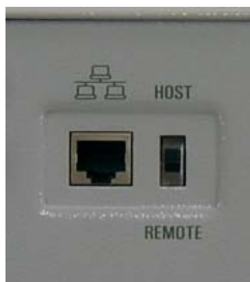
Figure 6 – Ethernet Port & Mode Selection Switch
