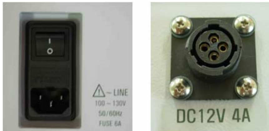
Figure 5 – Trilogue-1NM Repeater Power Switch
