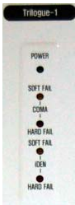
Figure 4 – Trilogue-1NM Repeater LED View
