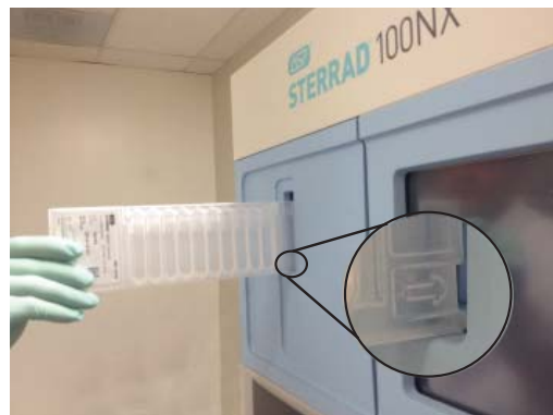
Figure 19b. Position the cassette so that the arrows are pointing straight into the cassette door slot of the sterilizer.
