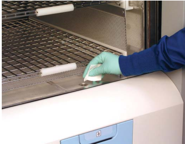
Figure 33. Cleaning the Hydrogen Peroxide Monitor Lens.
