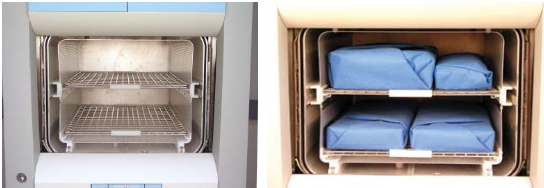
Figure 22. The STERRAD® 100NX® Chamber Empty and With a Typical Standard Cycle Load Correctly Placed.
