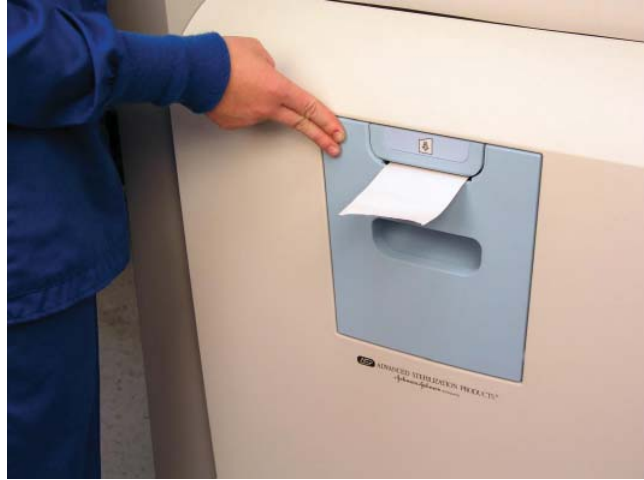
Figure 31. Make sure the Printer Door Latches Securely and the Paper is in Place.
