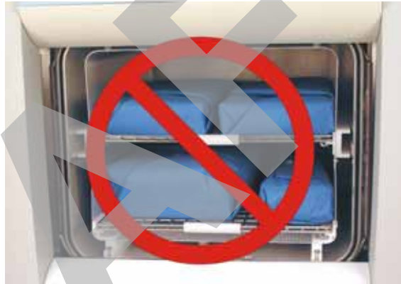
Figure 6. The Load Should NOT Touch the Electrode.
