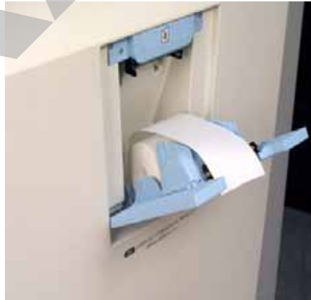
Figure 30. Insert a New Paper Roll.
