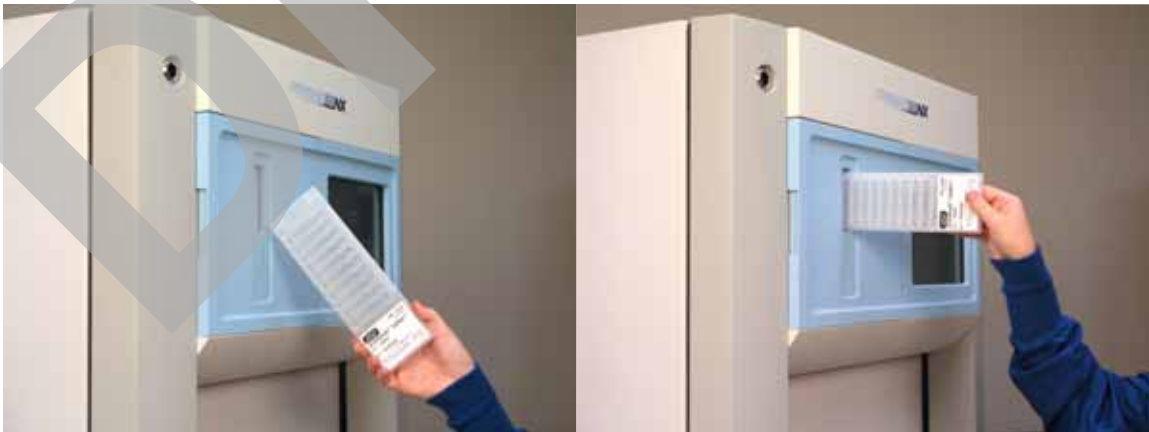
Figure 19. Inserting a Cassette.
