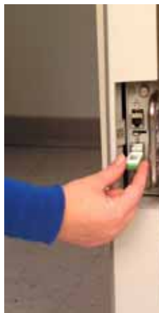
Figure 36. Insert the Memory Stick into The USB Port.
