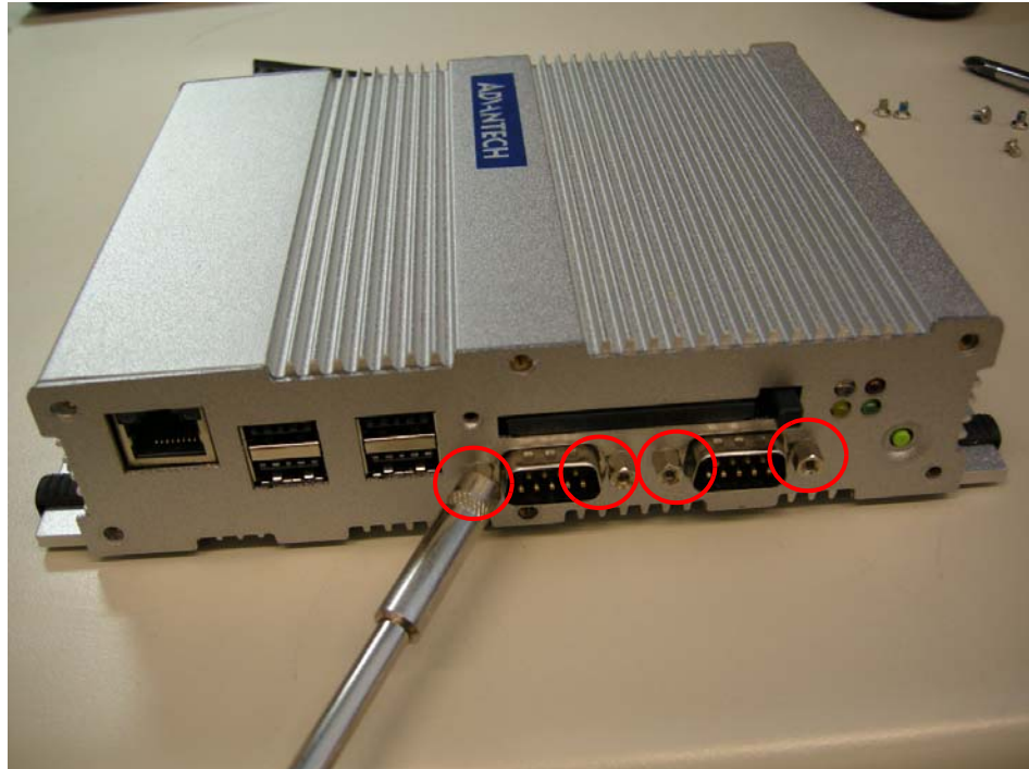
Figure 4.4 Unscrew the 4 Hex-bolt on the front face plate
