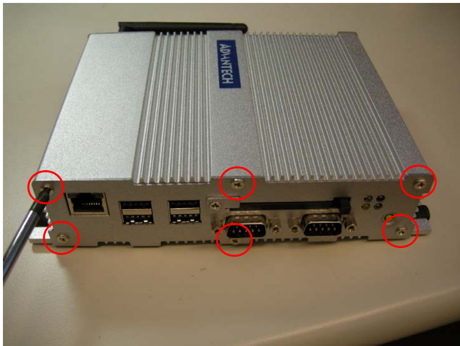
Figure 4.2 Unscrew the 6 screws on the front side frame
