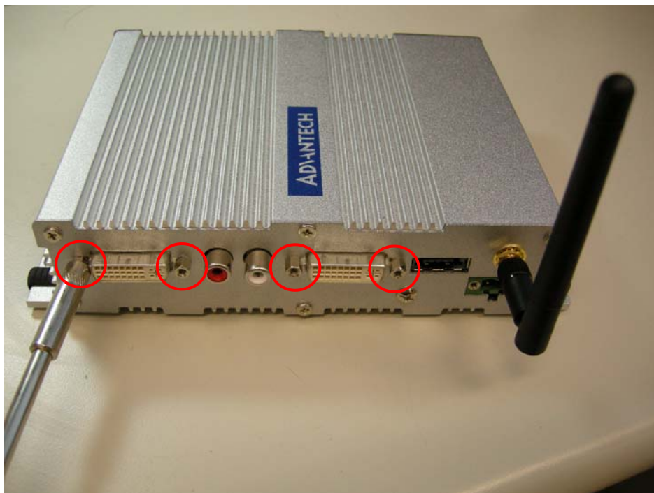
Figure 4.6 Unscrew the 4 Hex-bolt on the rear face plate
