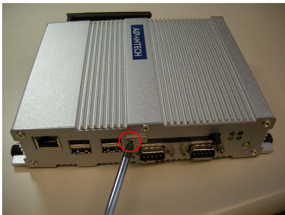
Figure 4.3 Unscrew the 1 screws on the front face plate
