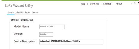
The screenshot shows the 'System' tab of the LoRa Wizzard Utility. Under 'Device Information', the following fields are visible: Model Name (WSW2C42100-1), Version (1.00.04), and Device Description (Advantech 4422E1D0 LoRa Node, 915MHz).
