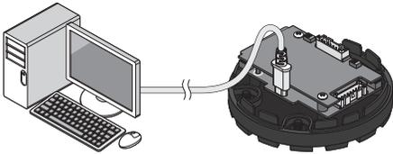
6. Once the device and computer are connected, the computer detects the USB connection and a virtual COM port is created.
