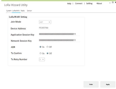
The screenshot shows the 'LoRaWAN Setting' page. Fields include: Join Mode (dropdown menu set to ABP), Device Address (FE2E2780), Application Session Key (00000000000000000000000000000011), Network Session Key (00000000000000000000000000000011), ADR (radio buttons for On/Off, with On selected), Tx Confirm (radio buttons for On/Off, with Off selected), and Tx Retry Number (dropdown menu set to 0). There are 'Undo' and 'Apply' buttons at the bottom.
