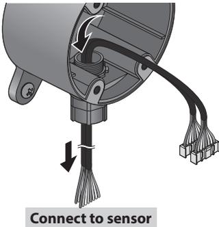
4. Connect the sensor cables to the connectors on the device.
