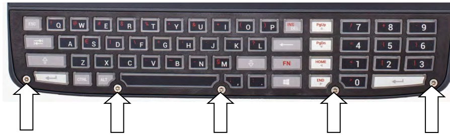
Fig. 16.1: Unscrew the mounting screws of the integrated keyboard
