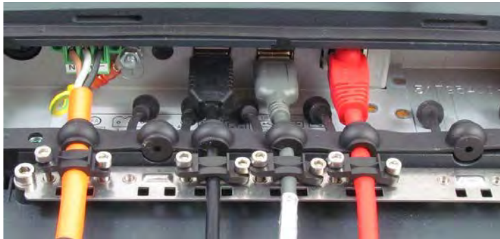
Fig. 12.6: Ethernet cable on the connector panel; secured to the strain relief rail
