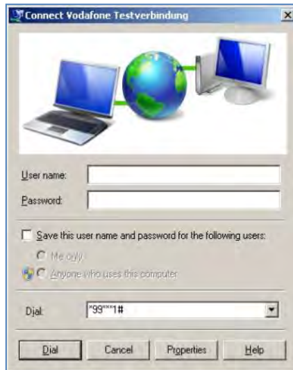
Fig. 10.20: QUECTEL EC25 - Dial Vodafone test connection
