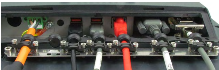
Fig. 12.7: COM cable on the connector panel; secured to the strain relief rail
