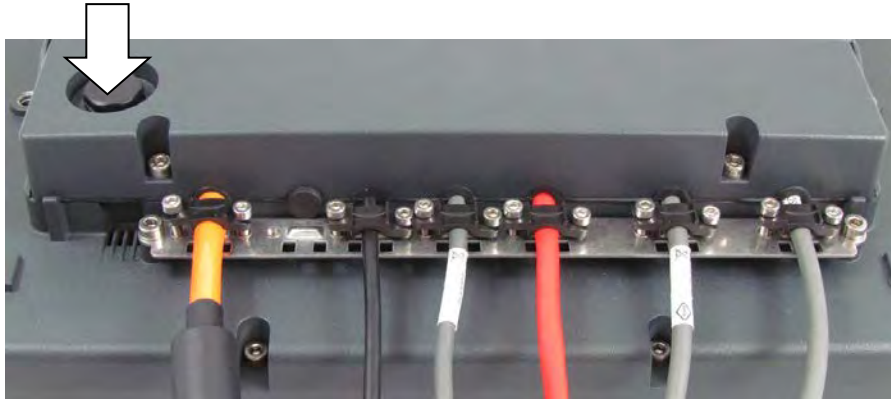
Fig. 12.10: Pressure compensation element - Do not modify or remove
