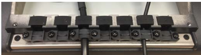
Fig. 6.1: Rubber seal inserted in the cable compartment
