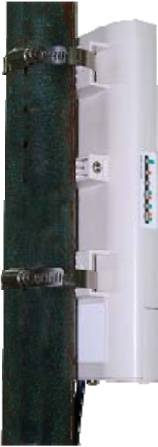
Figure 8 Pole Mounting – Step 2
