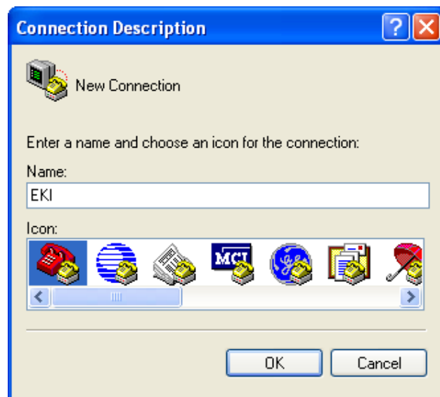
Figure 7.1 Creating a Telnet Connection
