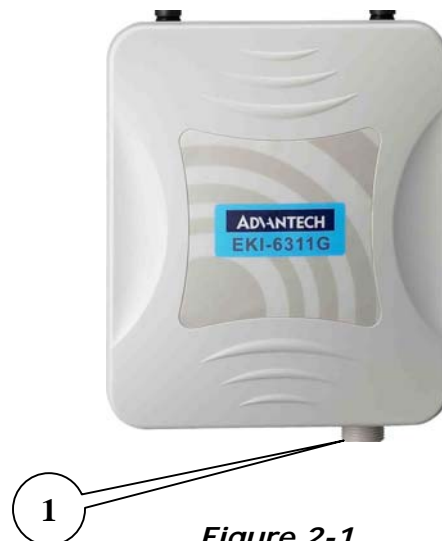
Figure 2-1 Power and Data Interface location on the PoE denoted by numbers 1-5.
