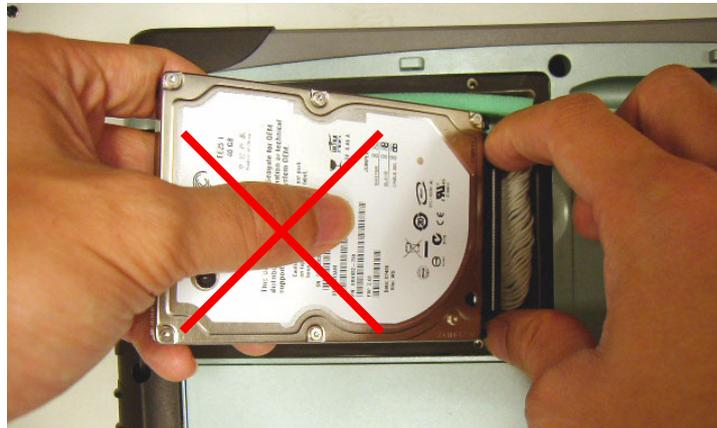
**Figure 4.6 Incorrect removal of the HDD**
