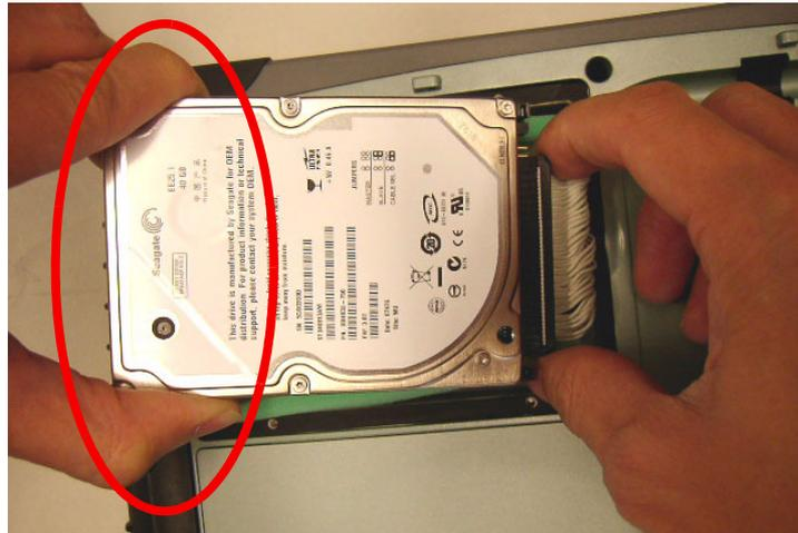
**Figure 4.5 Correct Removal of the HDD**
