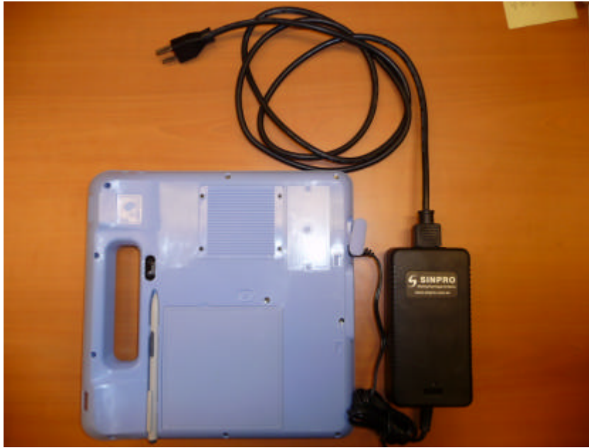
Figure 2-9: Connecting the AC Adapter power supplier with MICA
