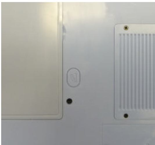
Figure 2-15: battery remove button of MICA
