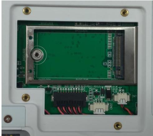
2. Insert the SSD, facing upwards, until it clicks into place. Screw and fix SSD
