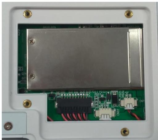
2. Unscrew and remove the shielding case
