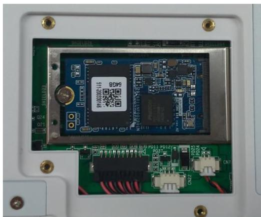
3. Unscrew and remove SSD from the slot.
