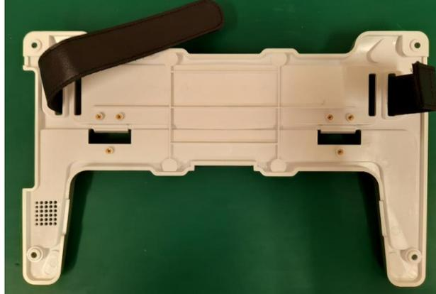
2. Pass the end of the hand strap through the inner hole on each side of the stand and stick the hand strap together
