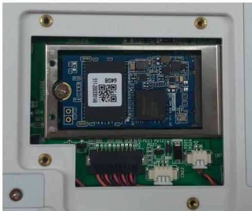
3. Screw and fix the shielding case.
