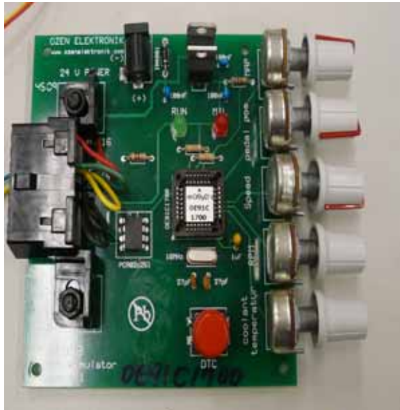
Figure 6.2 J1939 truck simulator
