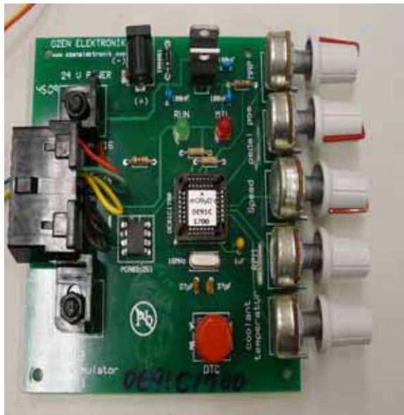
Figure 6.2 J1939 truck simulator
