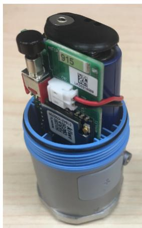
Figure 3.9 Battery Replacement Step 1
