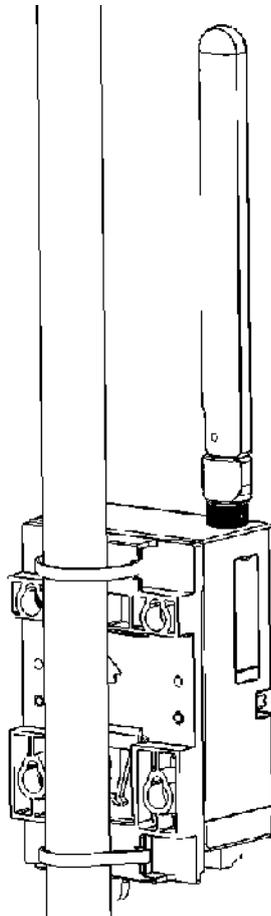
Figure 3.8 Pole Mounting Front
