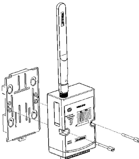
**Figure 3.3 DIN Mounting Install**
