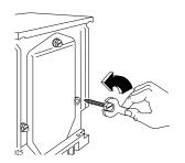
Remove the polystyrene block from the bottom of the machine and release the two plastic bags which are fixed under the filter door.
