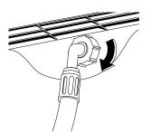
direction. Simply loosen the fitting, rotate the hose and retighten the fitting, making sure there are no water leaks.
