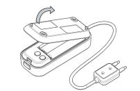
2. Remove the clear battery insulator by pulling it away from the Water Sensor
