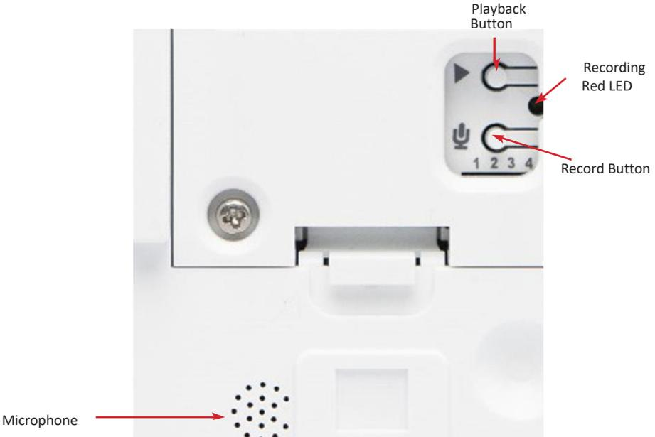
The Playback and Record buttons are found on the back of the monitor. The microphone is located outside the battery compartment as shown above.
