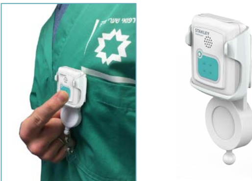
Figure 4: T14 Staff Badge Attached to a staff member's scrubs.
